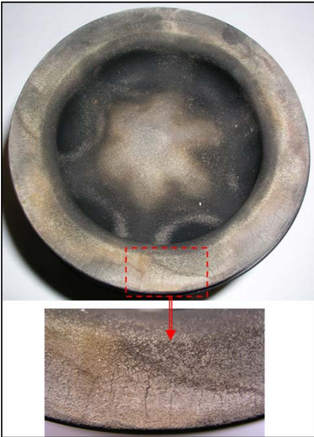
Fig. 6 Piston head after engine test with TBC coating showing soot and cracks
