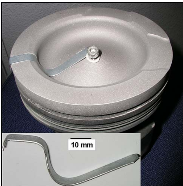
Fig. 1 Example of test plate used for coating thickness measurement
